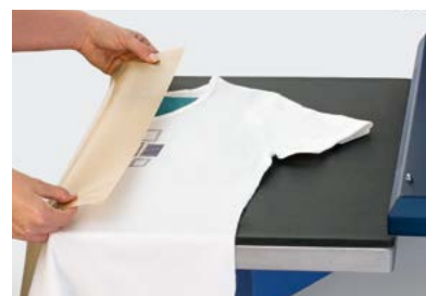
3 Make sure to apply the elements from the recommended side and use the correct pressurizing medium. To protect the heating surfaces from any glue residue, it is best to cover them with Teflon® foil.
