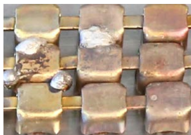
2 Too high temperature
