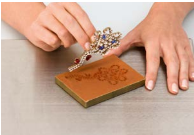
4 Once the material hardens, the original model can be removed.
