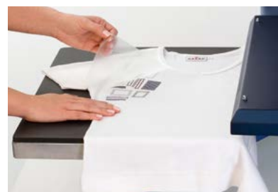
6 Once the product is at least hand warm, the transparent film can be removed at an acute angle*.
