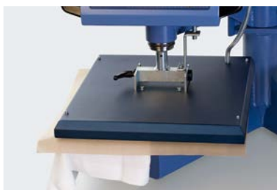
4 After pressure, time and temperature are set, close the heat press.
