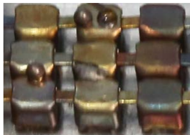
2 Too high temperature
