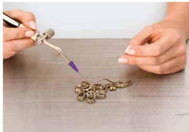
2 Strengthen the rear of the original model with wire.
